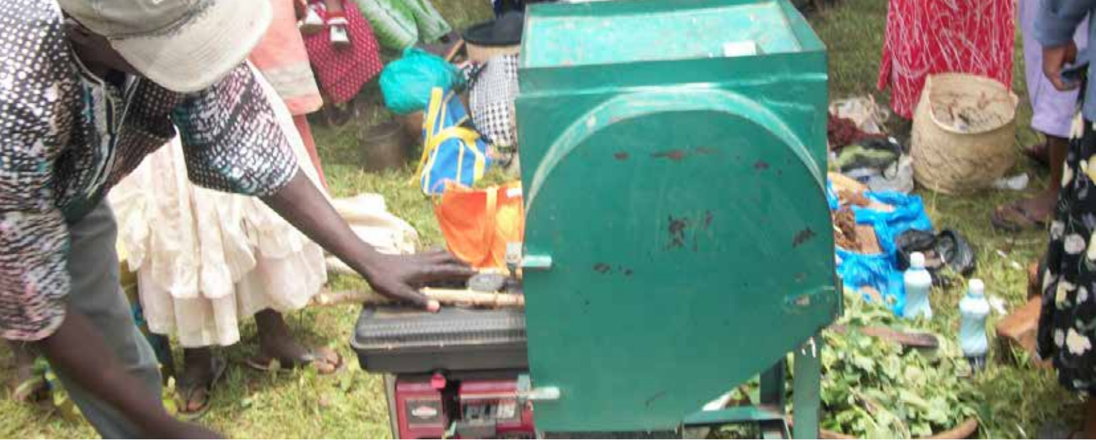
A manual thresher can be used to add value to vegetables, cassava, napier grass and any other farm produce
